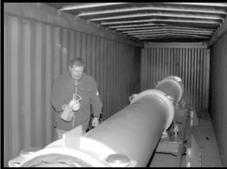
Checking in: A CERN technician inspects the superconducting magnet after arrival in a container from Brookhaven. The container is trucked to CERN, then lifted off the truckbed by crane and prepared for receiving.
