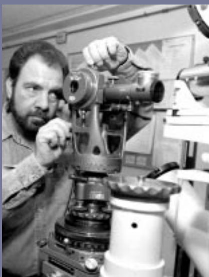
Ed Dijk sights through a gyrotheodolite, which uses an internal gyroscope to determine location on the earth's surface and the direction of true north.
