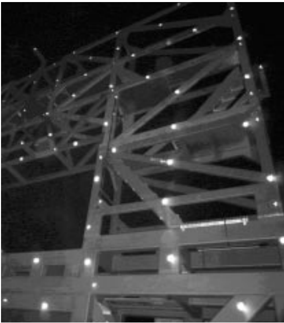
The V-Star targets light up the DZero end muon truss for three-dimensional coordinates.
