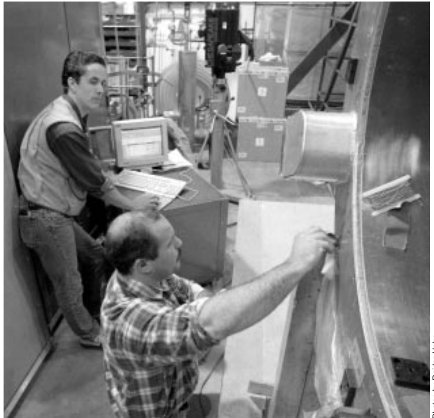
Mike O’Boyle (left) and Chuck Wilson attach tooling balls for use with a laser tracker, a “total station” device which gives coordinates in x, y and z planes.
