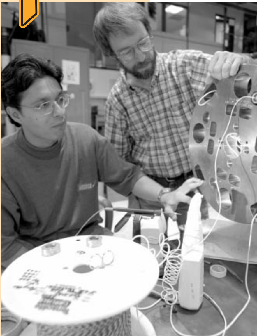
Engineers Tug Arkan (left) and Rodger Bossert examine the end structure of one of the final model magnets.
