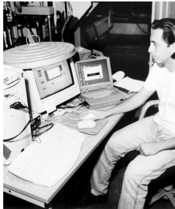
Graduate student Miguel Mostafa monitors the operation of the fieldmapper. The garbage can lid sitting on the computer serves as shielding against magnet flux from the detector.
