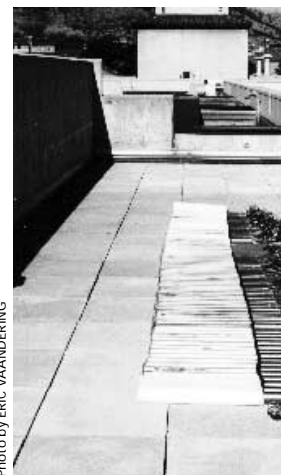
Elements of a lead-glass calorimeter arrayed on the roof of the physics building in Boulder. Glass that has suffered radiation damage (as part of a detector element in a previous experiment) can be cured by exposure to ultraviolet light, including sunlight.
