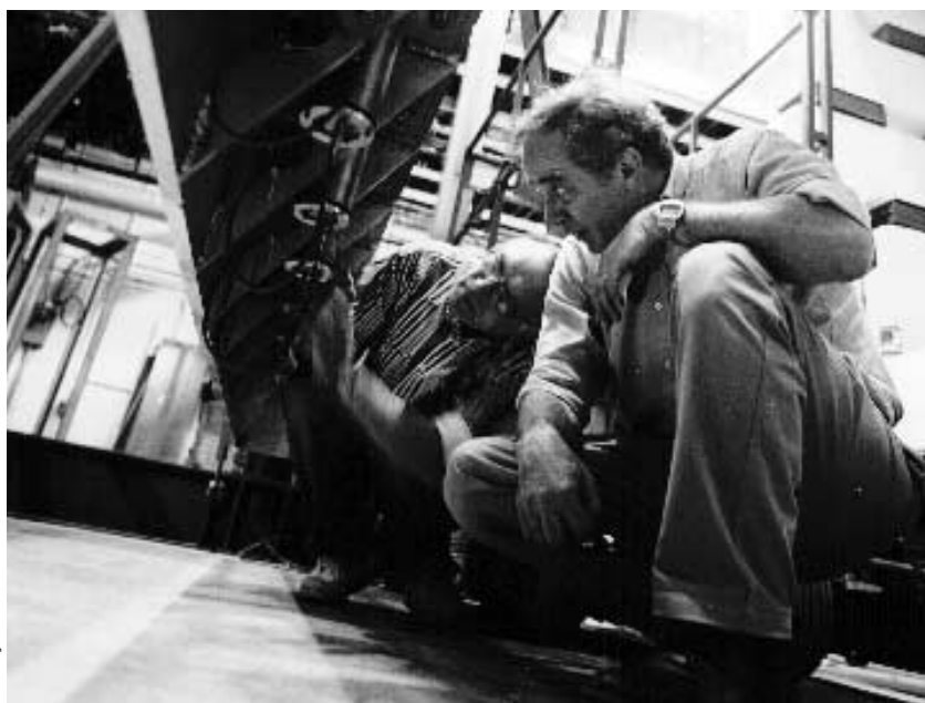
Uriel Nauenberg (foreground), CU physics professor, and Anatoly Ronzhin, guest scientist at Fermilab. They are checking the wiring of photomultiplier tubes at the base of a lead-scintillator calorimeter. CU students and faculty built the calorimeter in Boulder.
