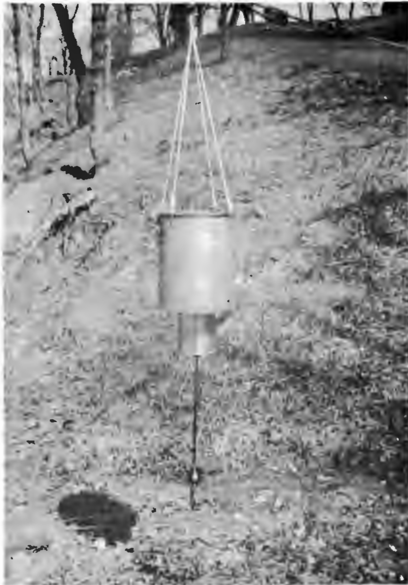
Figure 9 Fixed rate, manually operated ballast release assembly.
