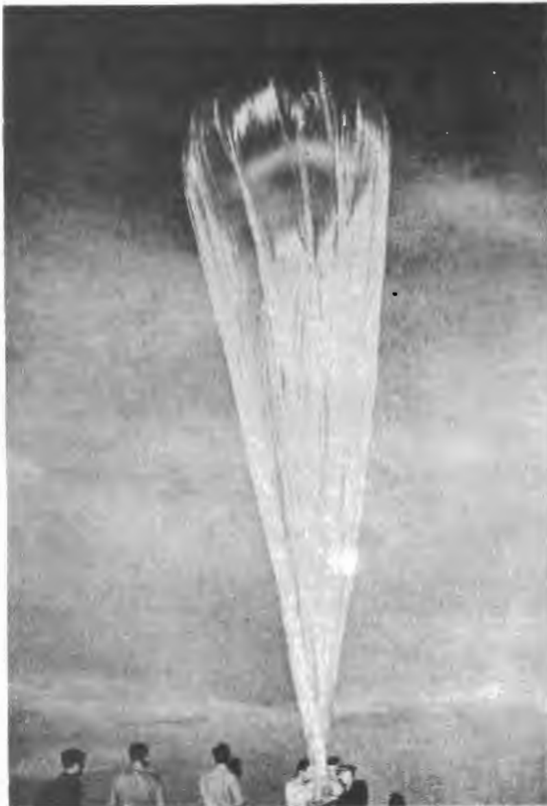
Figure 5. 20'-Diameter, teardrop polyethylene balloon. In all of these, film is .001" polyethylene, butt welded with fiber tape laid along the seams to reinforce the seal, and to carry
