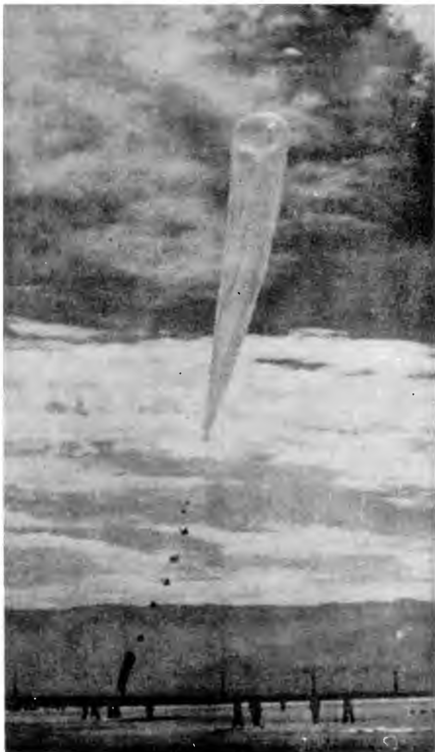
Figure 42 General Mills 70 foot balloon being launched in a 5 knot wind.
