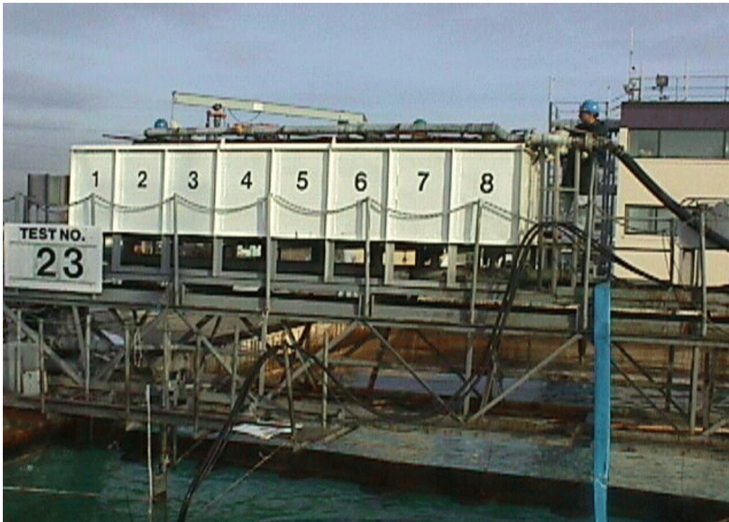
Figure 3 Oil recovery tank with eight cells on auxiliary bridge
