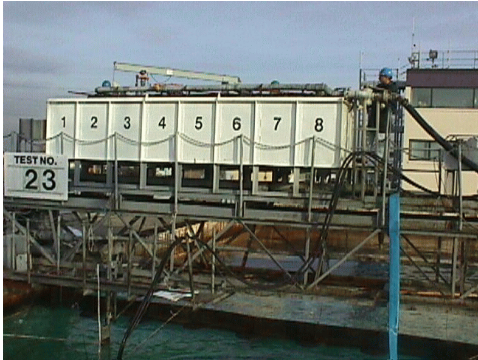
Figure 4. Oil recovery tank with eight cells on auxiliary bridge.
