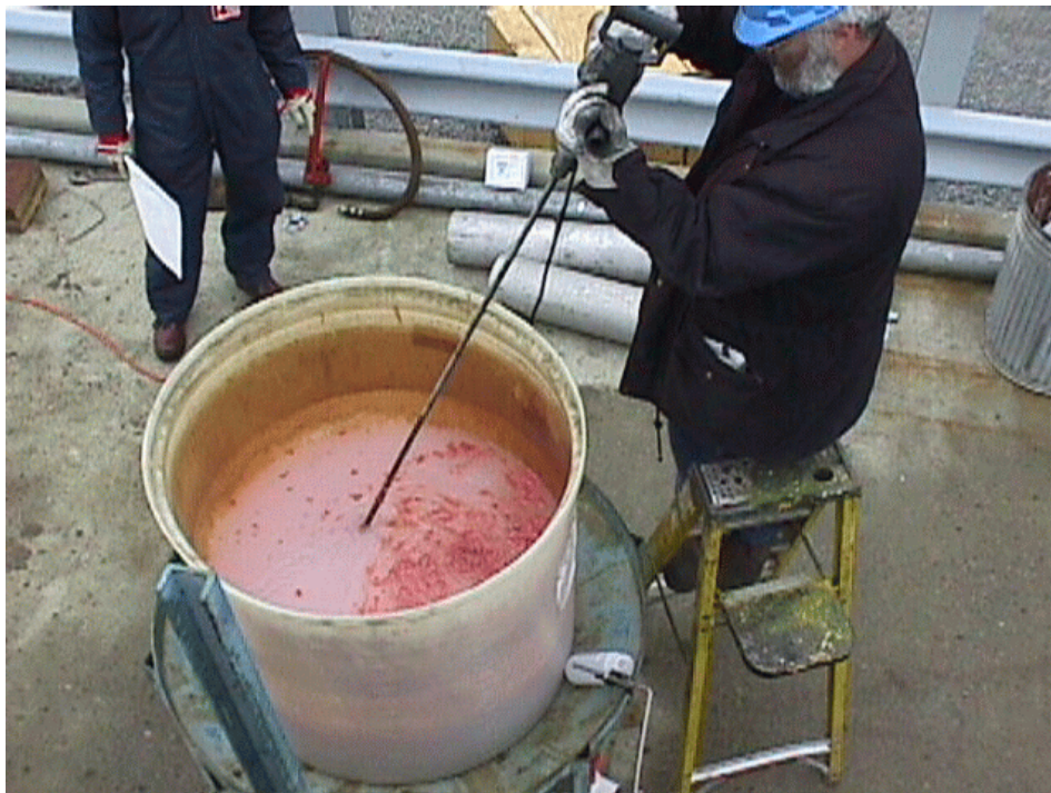
Figure 7. Stirring decanted water sample to obtain averaged sample for analysis.
