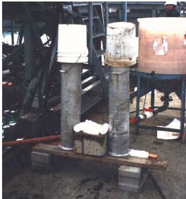
Figure 9. Steel columns used to hold 24-hour water samples (plastic buckets are to prevent rain entering tops)
