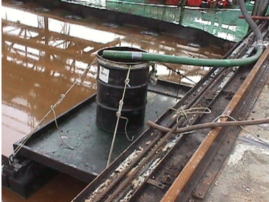
Figure 8. Skimmer discharging into a 55-gallon drum mounted on a raft to determine effect of waves on primary break time.
