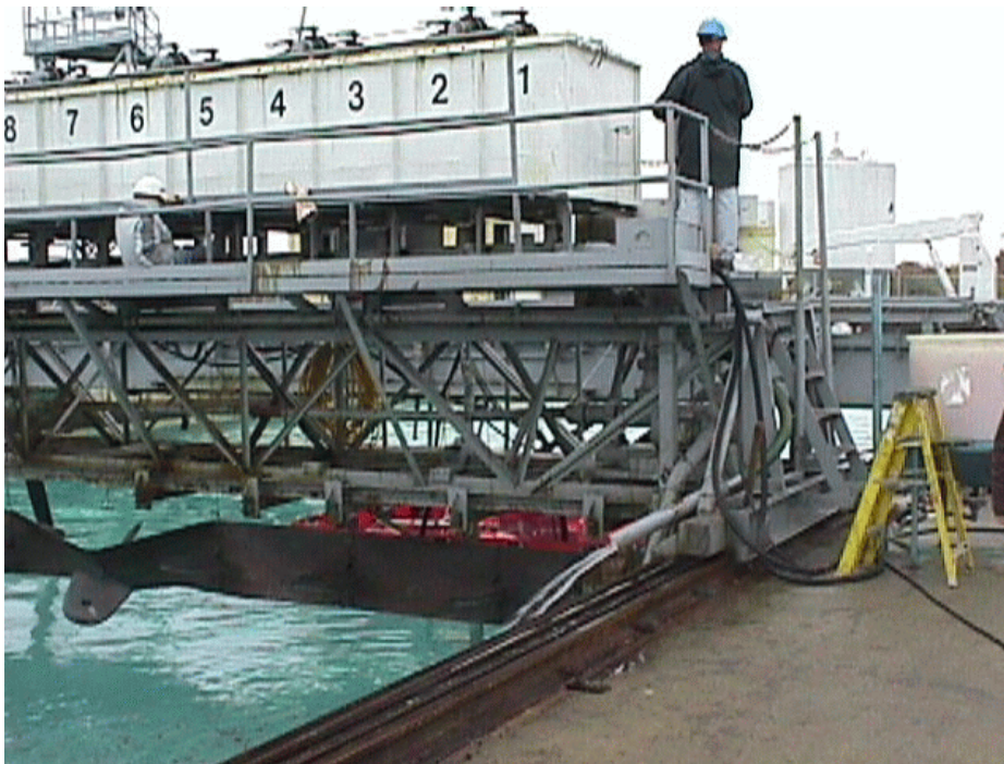
Figure 5. Decanting water from cell #5 back into test basin.
