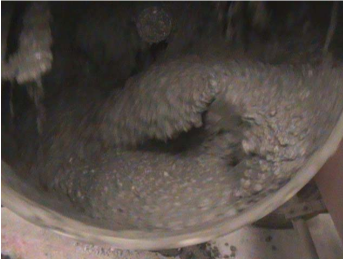
Figure 23: SCC rolling in the mixer
