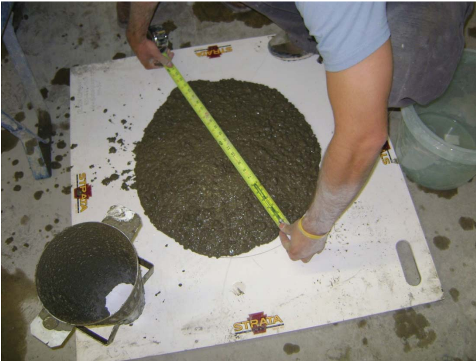
Figure 10: Horizontal measurement of slump flow
