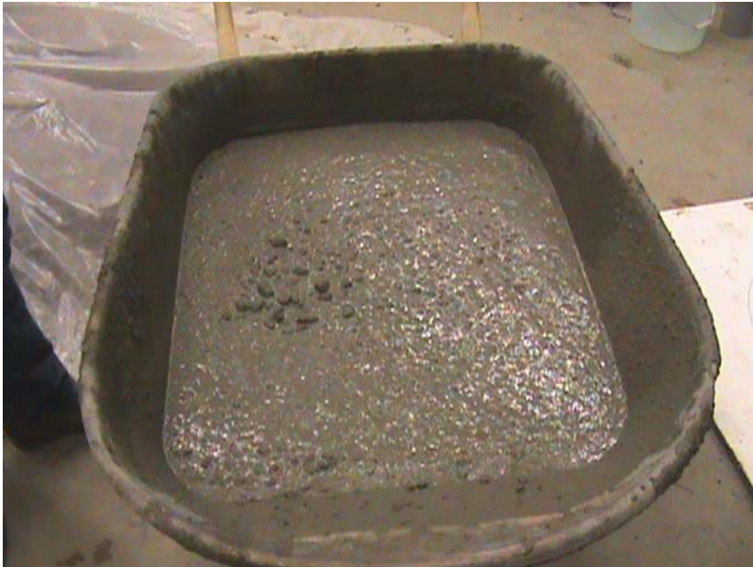
Figure 17: SCC:6.5:0.0:FA just prior to the spread
