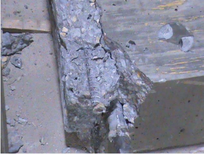
Figure 49: Aggregate distribution uniformity
