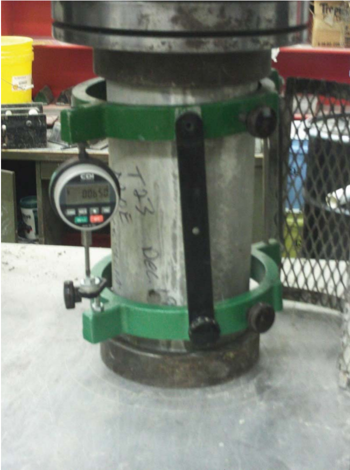
Figure 36: Modulus of Elasticity testing assembly
