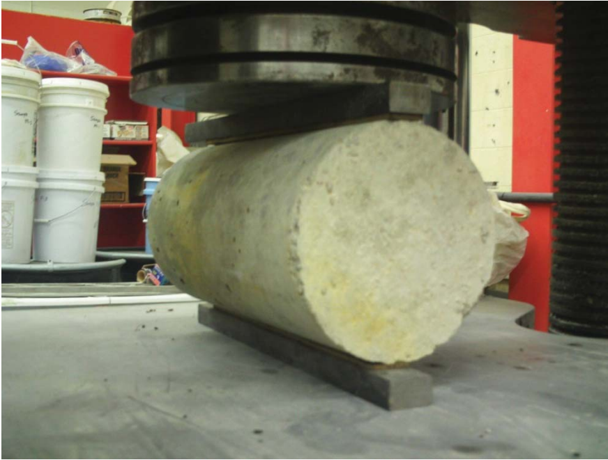
Figure 41: Splitting Tensile Test Setup.
