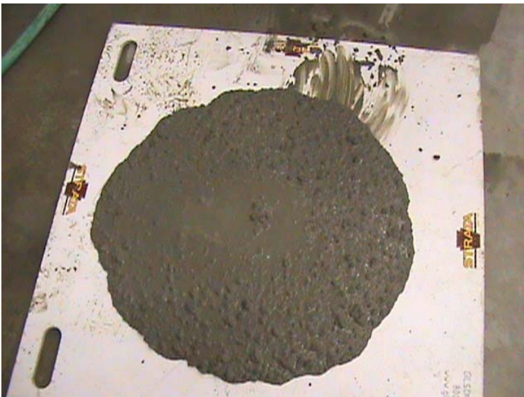
Figure 14: SCC mix with VSI=0.5, evidence of bleeding in the center
