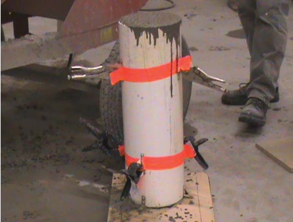
Figure 25: Column Segregation apparatus
