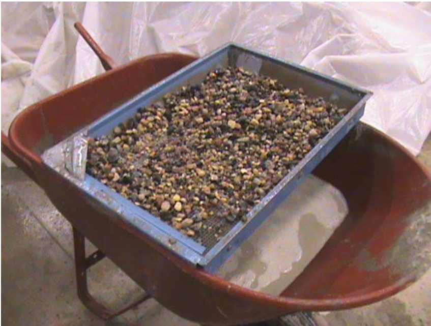
Figure 26: Aggregate washed over No. 4 sieve from the column segregation apparatus
