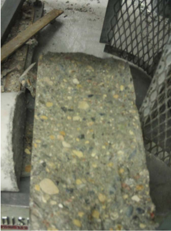
Figure 42: SCC specimen split after loading.
