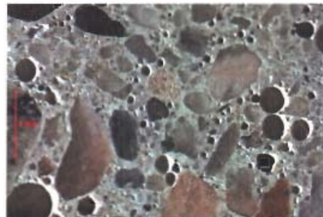
Magnification: 30x Description: Overall hardened air content, 5.4% total
