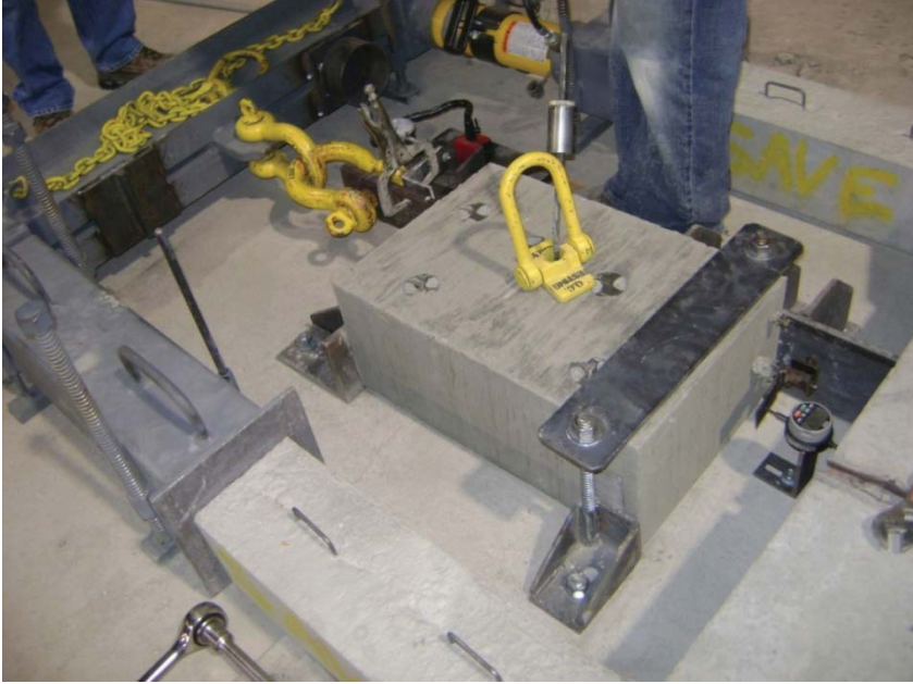
Figure 46: Slip measurement taken on the back side of the pull-out specimen
