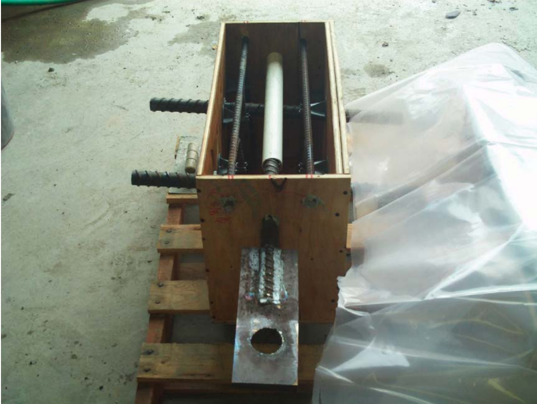
Figure 44: Pullout specimen before casting in concrete
