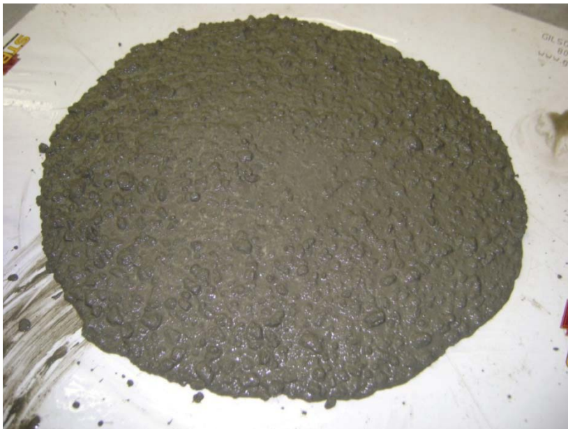
Figure 18: Spread of SCC:6.5:30FA with VSI=0, ideal spread
