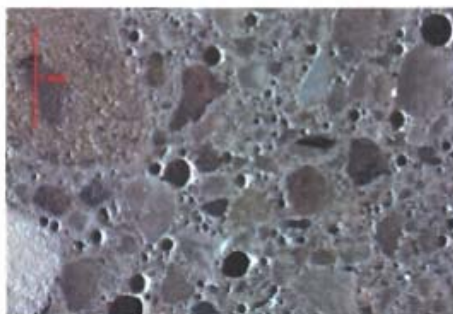
Magnification: 30x Description: Overall hardened air content, 4.6% total
