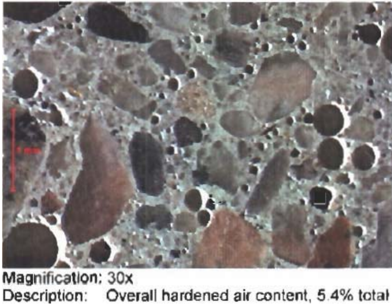
Figure 40: SCC:6.5:30FA, with spacing factor = 0.006"
