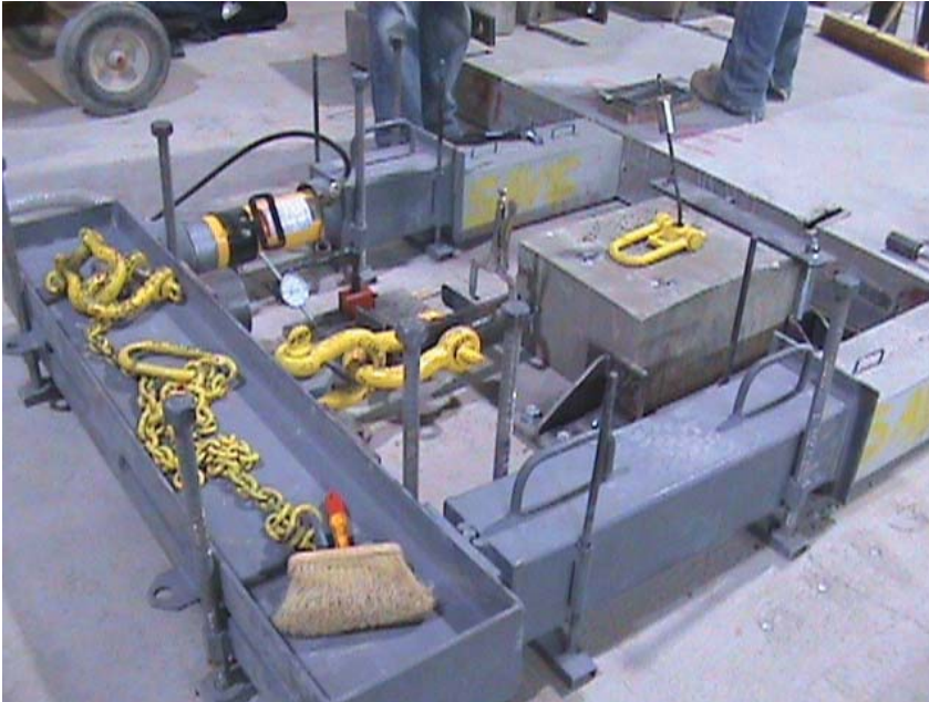
Figure 43: Pullout Test Setup.
