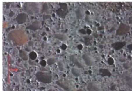
Magnification: 30x Description: Overall hardened air content, 3.5% total
