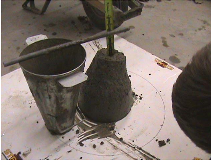
Figure 12: Slump of NC mixes varied between 3 inches and 4 inches, see Table 9 and Table 12.
