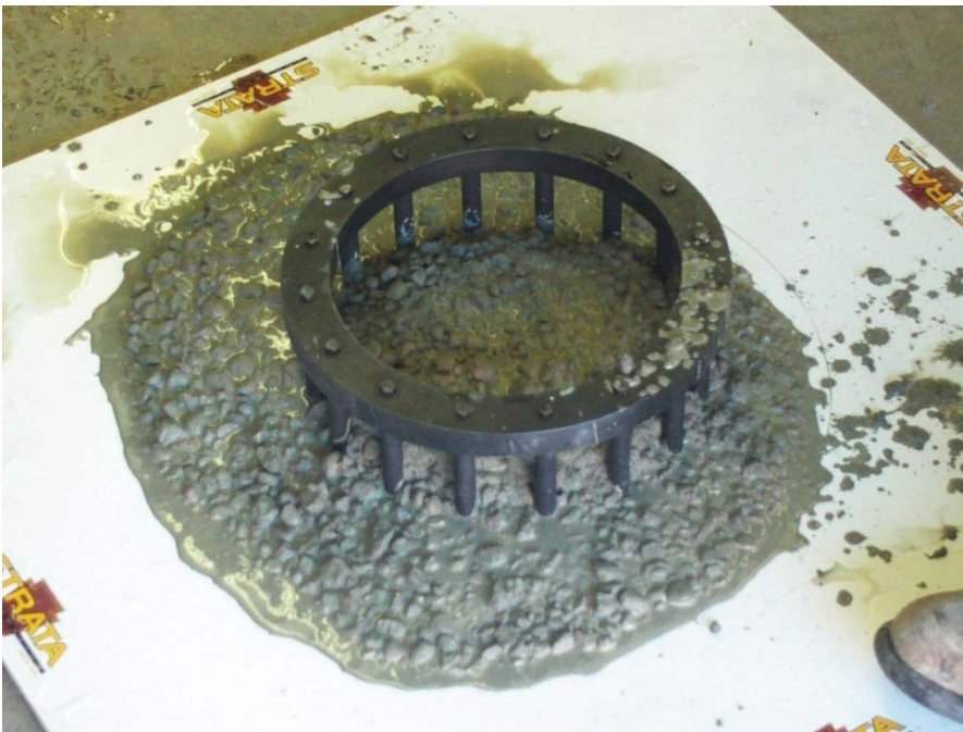
Figure 21: Slump flow with J-Ring VBI = 3.
