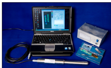
ProxiScan™ consists of a prostate probe, an external surge box, and a computer.
