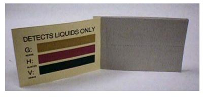
clothing or place it on a surface so it can be exposed to drops of liquid splash of chemical agents. If colored spots appear, chemical agent is present. Put on protective mask. Compare colored spots with colors on inside cover to determine type of agent. The paper may also be used to detect liquid contamination by placing the paper in contact with the suspected surface.
