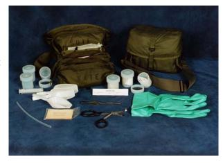
and/or surface samples. The kit contains Teflon containers and expendable materials for taking 2-3 of each type of sample. The jars are capable of containing chemical agents at high (120° F) and low temperatures. Other components in the kit include gloves, tweezers, syringes, scoops, and M8 Detector Paper. Samples are labeled and packaged, along with identifying documentation, for transport.
