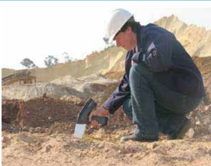
The Innov-X System pictured here being used, is a handheld elemental analyzer for detecting metals. Innov-X System received an investment from CEI Ventures, Inc. (CVI). TD Banknorth is an investor in CEI Ventures, Inc.
