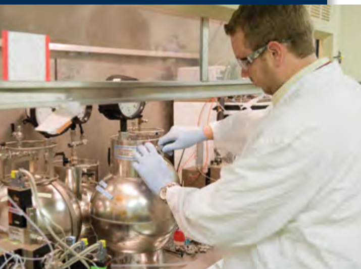
Principal Investigator Greg Peterson sets up a micro-breakthrough test system in order to determine the chemical capacity of a ZZAT variant.
