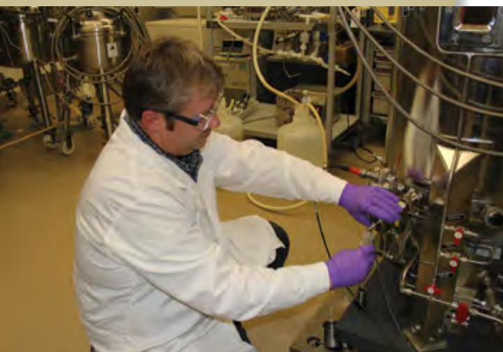
Research Biologist Joe Kragl, with the BioSciences Division, samples barcoded Bacillus thuringiensis spores during fermentation.
