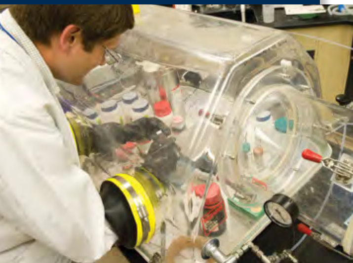
T. Grant Glover, Ph.D., (ECBC-SAIC) works with air-sensitive materials in a glovebox, synthesizing candidate novel materials for use in filters.
