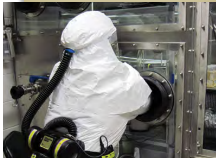
A researcher assesses a sample inside a glovebox, a sealed environment within the BSL-3 laboratory
