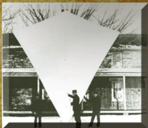
In 1895, Lt. Hugh D. Wise experimented with photo kites at Madison Barracks, N.Y. He built a kite 18 feet high and attached a box camera to it with string. Triggered by a timing device, the camera took photos from an altitude of 600 feet.
