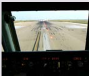
RWSL systems are fully automatic and designed to reduce the number and severity of runway incursions.
