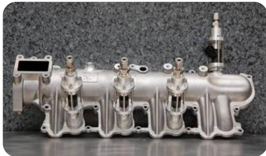
Modified Intake Manifold with PFI Injectors
