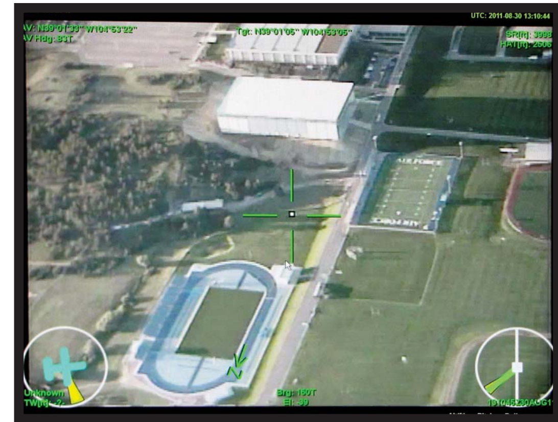
The Aerosonde Mk IV features a continuous zoom, electro-optical and imaging infrared camera. The aircraft can fly continuously for up to seven hours.
