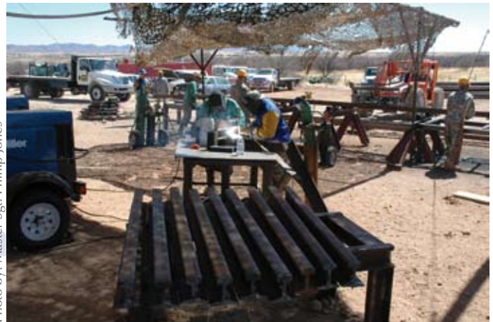
The 122 nd Engineers vehicle barrier fabrication yard near Sasabe, Arizona was a very active location as recycled railroad rails used in the 19 th century were cut into main-beams, cross-beams and keys; then assembled, transported and placed into position by 122 nd Soldiers along the U.S. - Mexico border.
