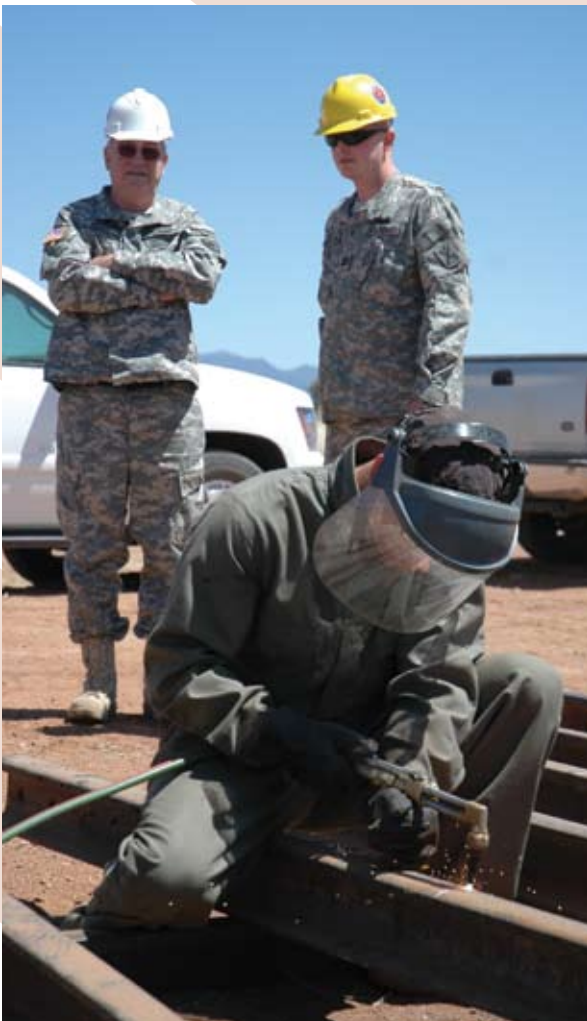
(L-R): Pfc. Jonathan Robeson of Spartanburg (center) cuts recycled railroad rails for use in constructing cross-beams for transportable vehicle barriers as Maj. Gen. Spears (left) and Capt. Simon Stricklen of Welford (right) observe.
