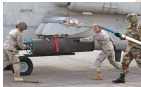
After loading the 30mm guns, Hydra rockets are loaded for firing. An Apache can hold 19 rockets on each side of the aircraft, for a total of 38. (Photos by Master Sgt. Philip Jones)
