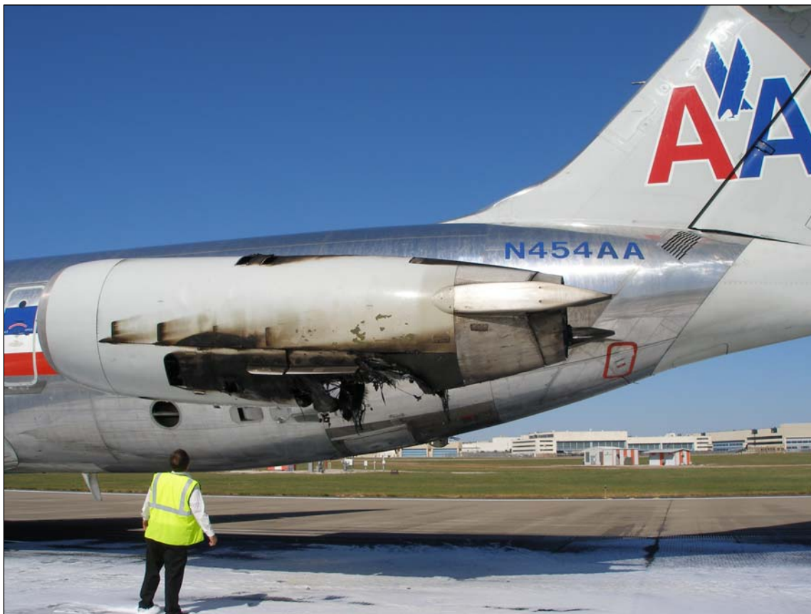
Figure 1. Photograph of the left side of the airplane after fire-extinguishing efforts were completed.
