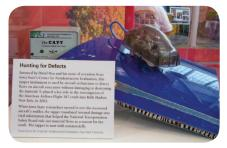
Equipment capable of testing aircraft components for structural flaws without damaging or destroying the part being tested is now available commercially thanks to research at Ames Laboratory.
