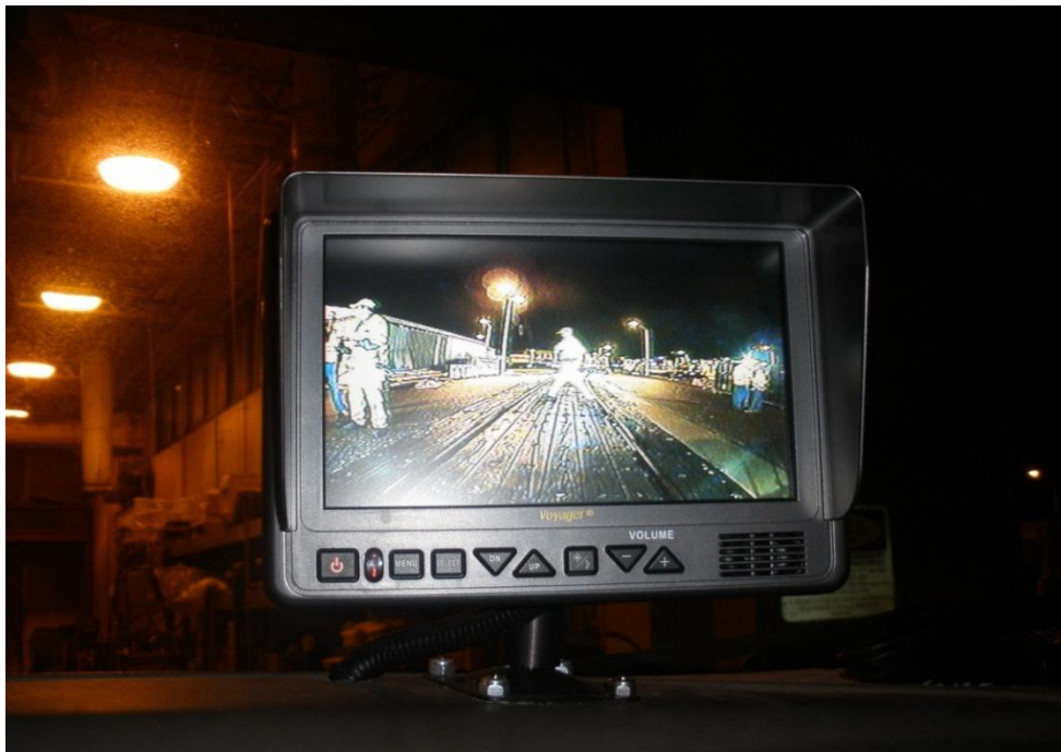
Figure 7. Video screen for backup movements in a hi-rail vehicle retrofitted with the upgraded lighting package.
