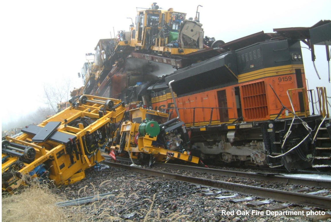
Figure 6. Wreckage including lead locomotive of striking train.
