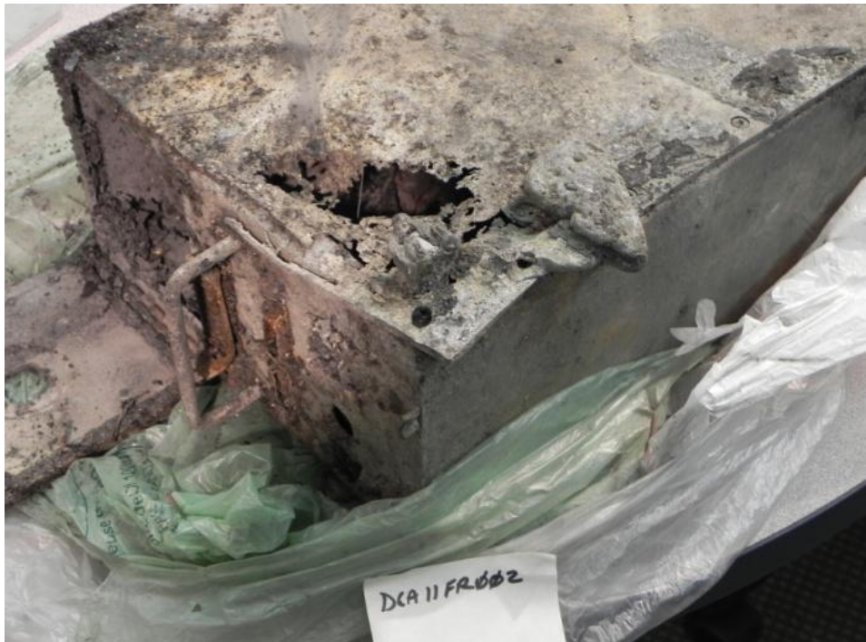
Figure 21. Fire-damaged video recorder hard drive enclosure from BNSF 9159.
