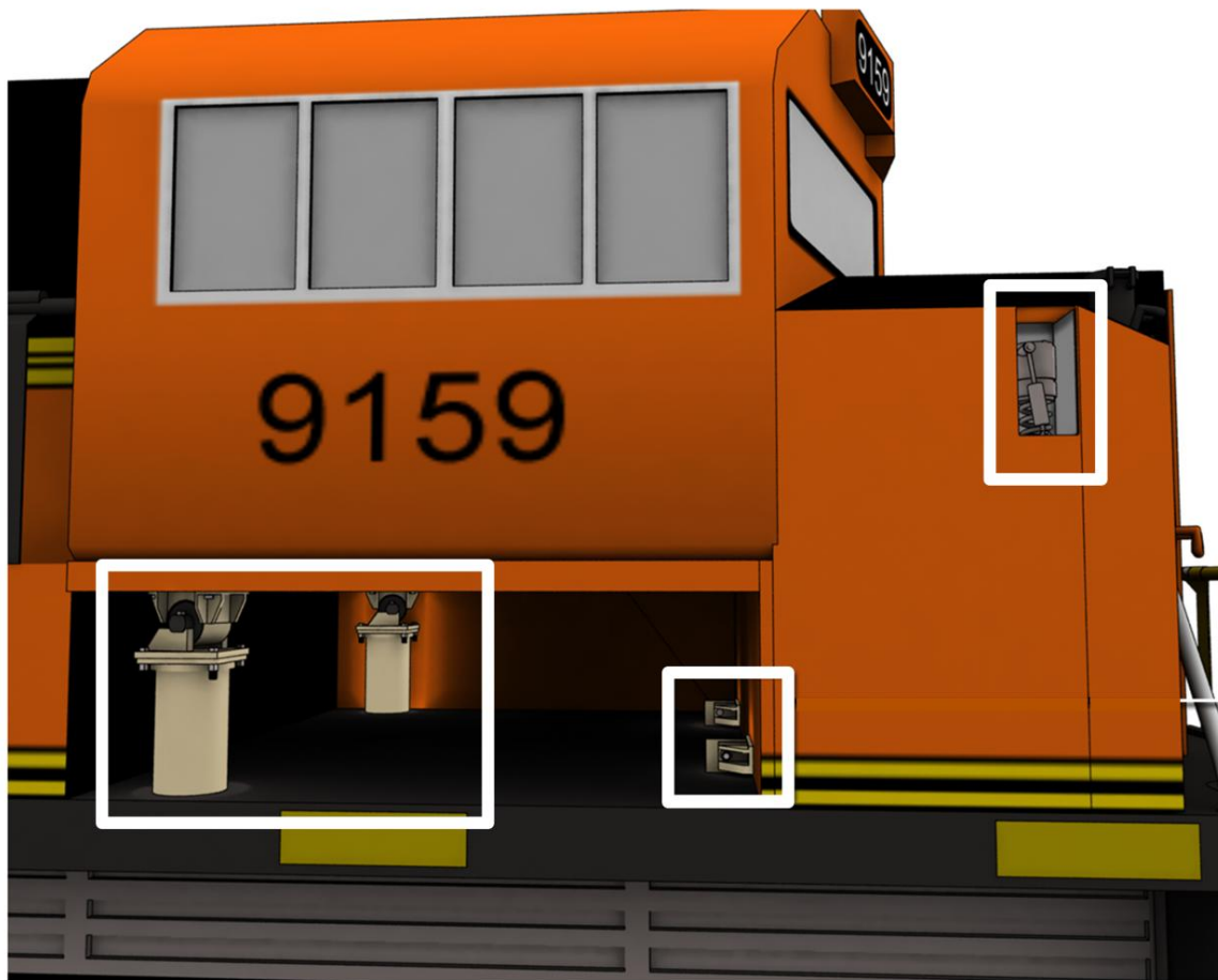
Figure 14. Illustration of EMD SD70Ace locomotive (same type as striking train locomotive) with white boxes indicating the points where the isolated cab attaches to the underframe.
