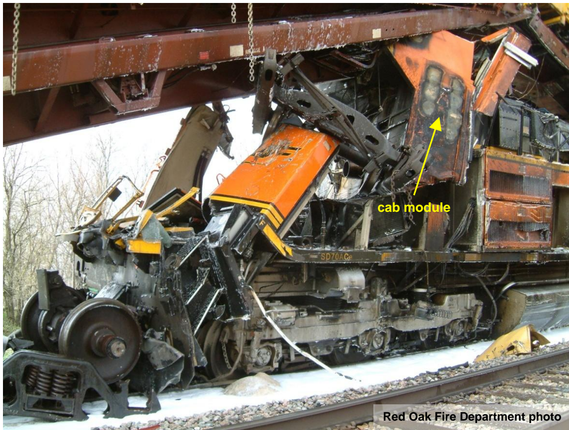
Figure 11. Upended striking train locomotive (BNSF 9159) modular operating cab.
