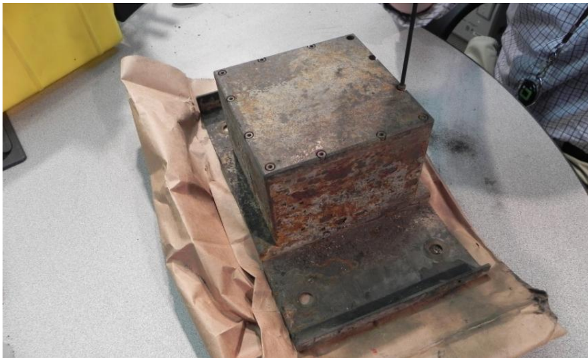
Figure 19. Fire-damaged memory module recovered from BNSF 9159.
