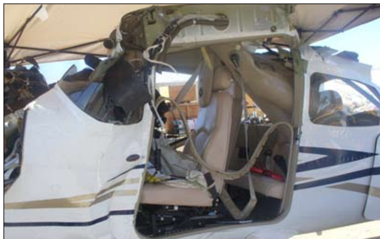
The main cabin portion of a Cessna 172S that crashed in Fullerton, California, on September 30, 2008 (LAX08FA301). The deployed airbag is resting on the front left pilot seat.
