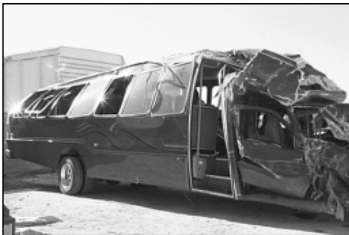
Body damage to nonconforming bus involved in the San Miguel accident.
