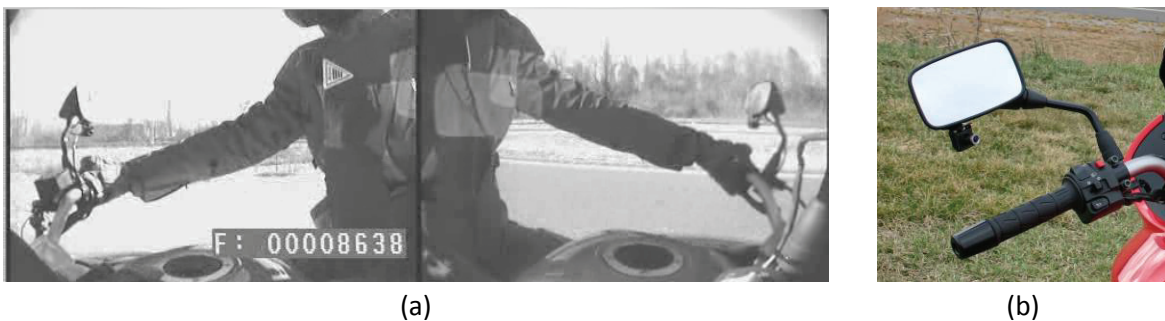
Figure 6. Side-view camera Configuration #1 with mirror mounted cameras facing across the bike.
