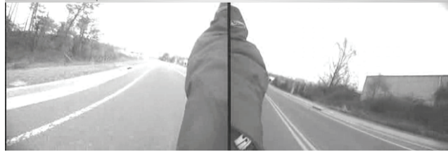
Figure 7. Side-view camera Configuration #2 with mirror-mounted cameras facing rearward.
