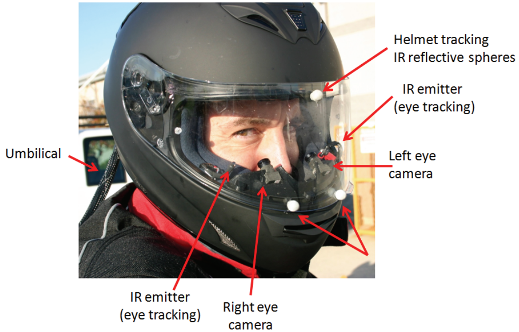
Figure 26. Helmet-mounted eye-tracking system and reflective markers.
