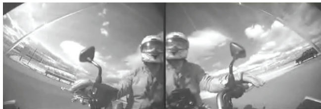
Figure 8. Configuration #3 -- Centrally mounted side-view cameras.
