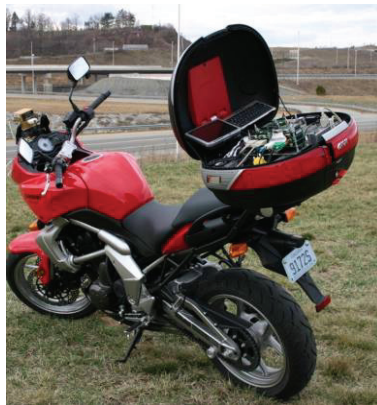
Figure 1. Main DAS unit – carry-over components.
