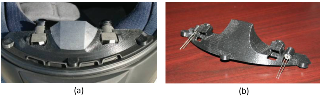
Figure 24. Fabricated fog-shield mounts for ocular cameras.
