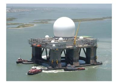
The Sea-Based X-Band Radar, seen here following initial sea trials, will provide the Ballistic Missile Defense System with a missile tracking and discrimination capability that can be positioned to cover any part of the globe to support both missile defense operations and testing.
