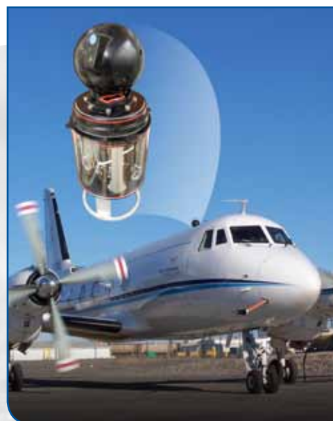
The 4STAR instrument (inset) is installed through the upper hull of the G-1 research aircraft.
