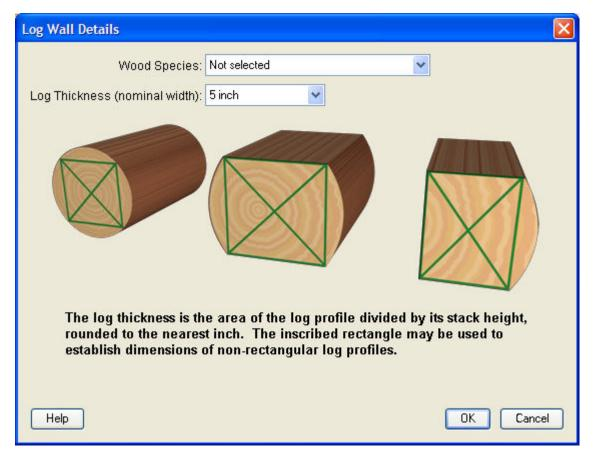
NOTE: Concrete, masonry, and "qualifying" log walls receive a mass wall credit in some locations. In order to qualify for this credit, the heat capacity of the exterior wall must be greater than or equal to 6 Btu/ft² °F [123 kj/m² °K] of exterior wall area. Masonry and concrete walls having a mass greater than or equal to 30 lb/ft² of exterior wall area (146 kg/m²) will meet this requirement. Masonry and concrete
