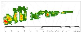
The 1:1,000,000 RIP Tool probability contour (light blue line) compared to grid output for one lane on the MF-2 range at Schofield Barracks, Hawaii. The grid data ranges from low probability of ignition (green) to high probability (red). Grid data outside of the contour has a probability of less than 1:1,000,000.
