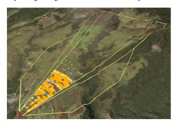
Real-world test of the prototype RIP Tool on the MF-2 Range at Schofield Barracks, Hawaii for 5.56 mm M856 tracer ammunition. The area affected by potential ignitions according to the RIP Tool (orange) is 3.2% of the size of the bat wing SDZ (yellow line). Red points are firing points and X's are targets.
