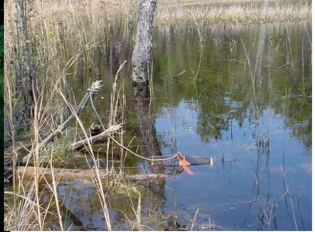
Minnow trap set in shallow wetland at Camp Lejeune. Note that the trap is set with the top above the water line and is tethered and marked with flagging.
