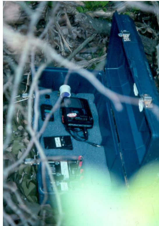
Portable FrogLogger; the microphone that extends from the upper end of the box is placed inside a cut-off 2-liter bottle for protection from weather, tied to a limb, and directed toward the pond.
