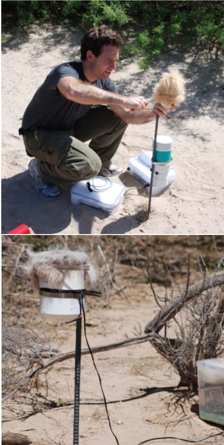
Two types of autonomous recording units (ARUs), as deployed in the desert north of Yuma, AZ in spring 2007. a) CLO BIN-file ARU with external microphone and battery packs. b) mp3-file ARU with mp3 player (bottom right) and battery pack.
