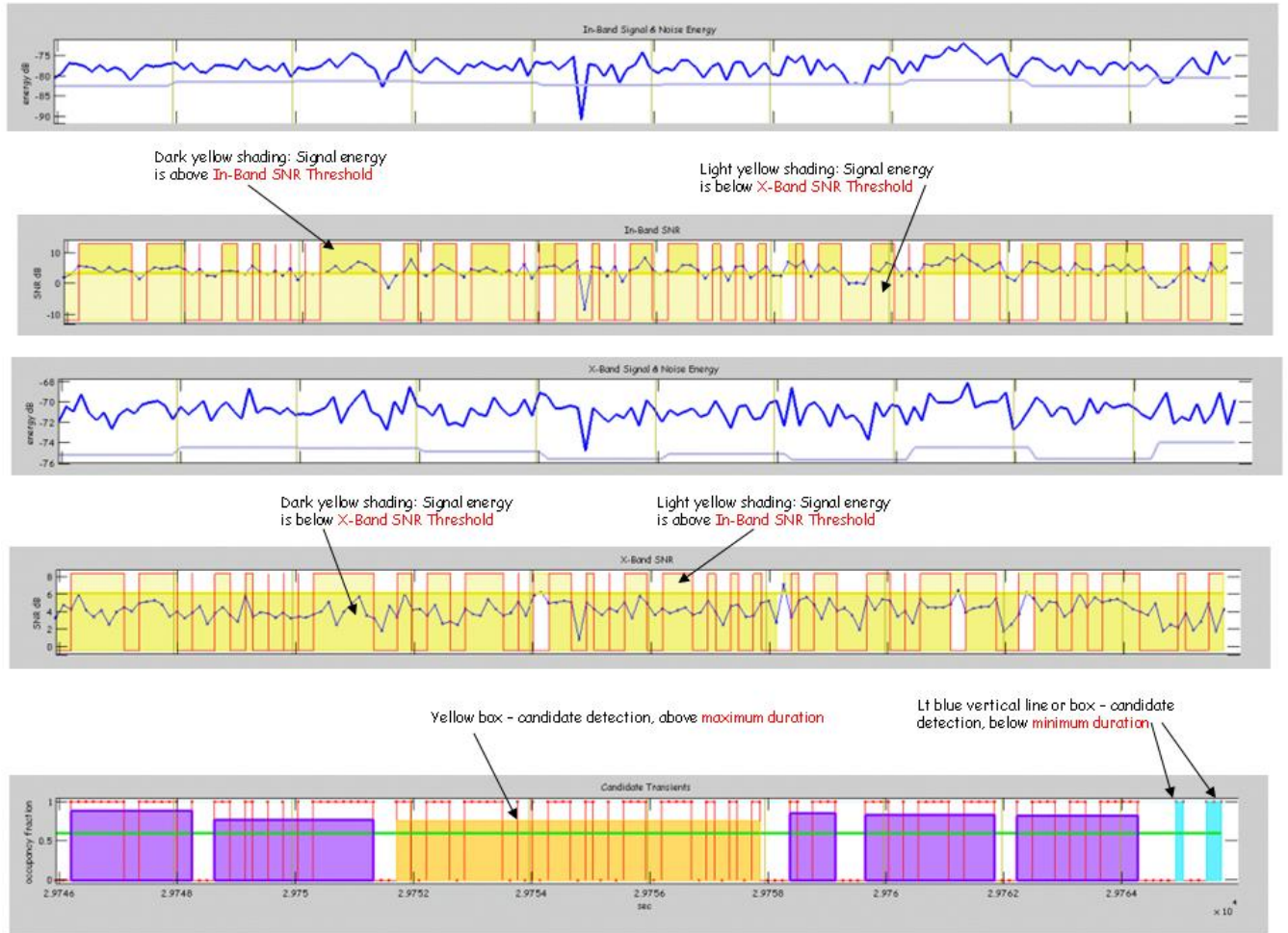
Figure 5b. Diagnostic tool definitions. Each definition represents a parameter setting in the dialog box to set energy detector algorithm settings for automated detection; however this figure contains an exclusion band setting, which allows the user to exclude signal energy in frequency bands outside of the band of interest for detecting flight-calls.
