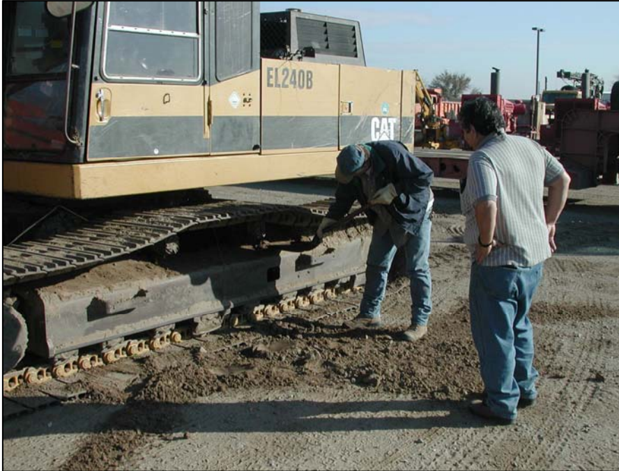
Figure 7. Precleaning heavy accumulations can help reduce water use when washing (photo courtesy of Fred Nibling).
