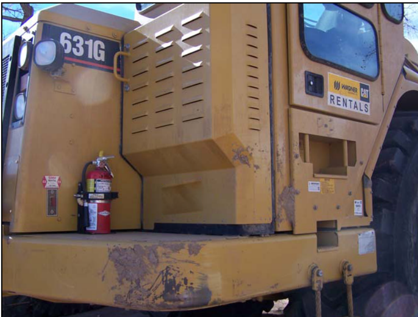
Figure 8. Rental equipment may be delivered to a worksite with mud accumulations. Consider including equipment cleaning in the equipment rental contract (U.S. Army Corps of Engineers photo).
