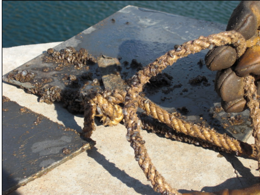
Figure B-13. Antifouling coating test panel has been in the Lower Colorado River at Parker Dam for 4 months; notice the attached adult quagga mussels on the test panel and anchoring ropes (photo courtesy of Joe DiVittorio, 2008).
