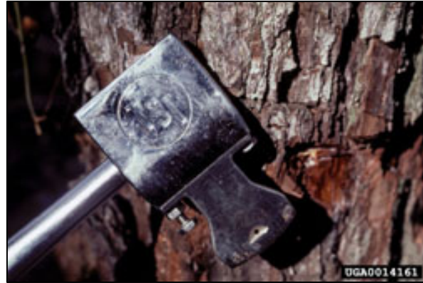
Hypo-Hatchet® showing hole in bit where herbicide is injected. Photo by Gerald Pearce, BUDWASH.org
