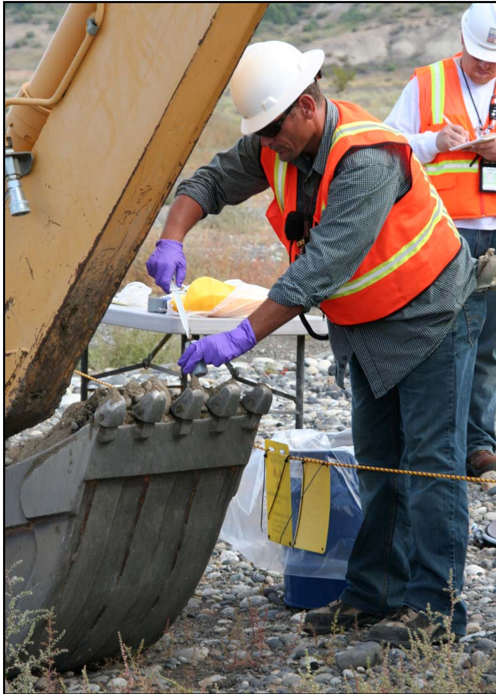
Samples are taken from the excavator bucket at site 100-F-26:4.
