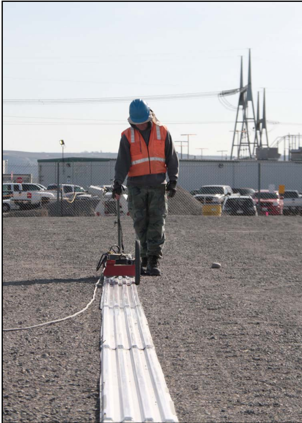
A worker from Sage Earth Science performs geophysical delineation at the 618-11 Burial Ground. Washington Closure Hanford soon will begin in situ radiological characterization of the burial ground's vertical pipe units. (Photo 9)
