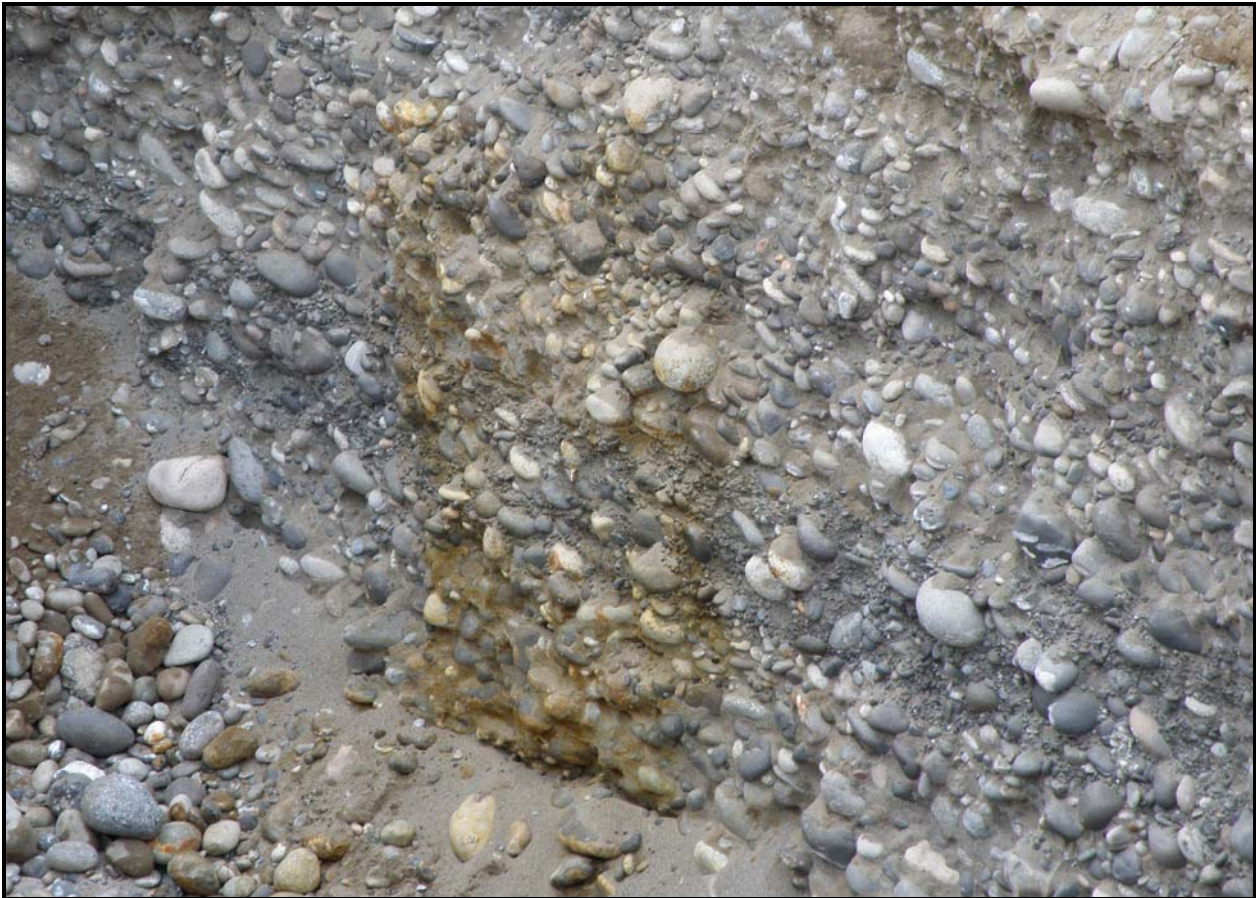
The stained side of a test pit at 100-F-57, where hexavalent chromium was found. (Photo 8)
