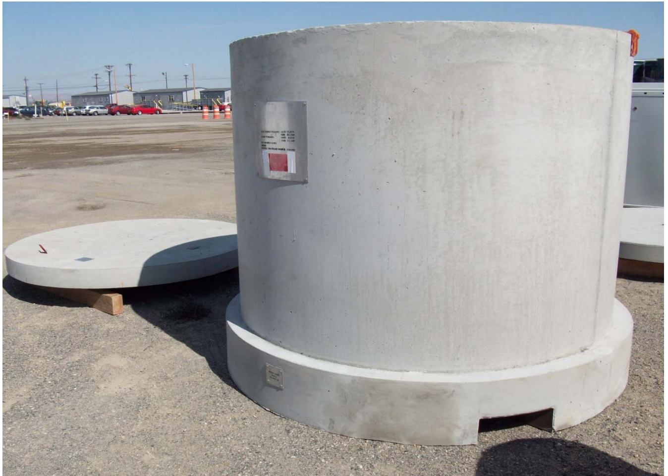
One of the first of 21 concrete shielded overpack containers that arrived last week. The overpacks will hold high-dose rate containers.
