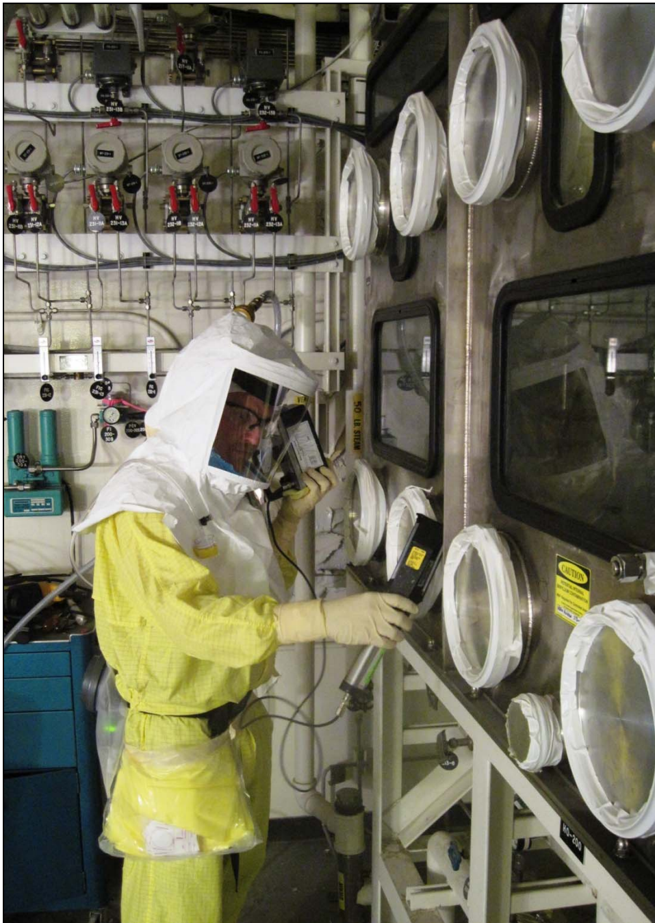
A radiological survey is performed on a glove box in the 209-E Criticality Mass Laboratory. Equipment like glove boxes must be removed from the facility before it can be demolished.
