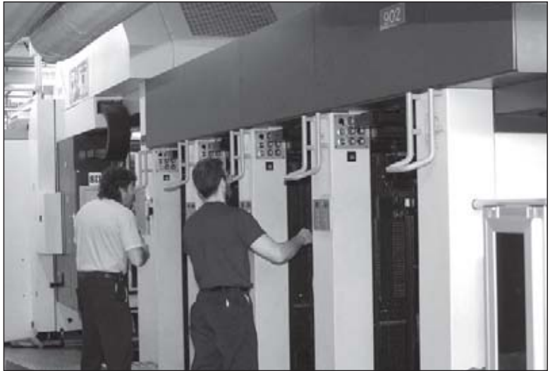
Plate printers Richard Zachmann and Jose Del Toral operating a new intaglio printing press.
