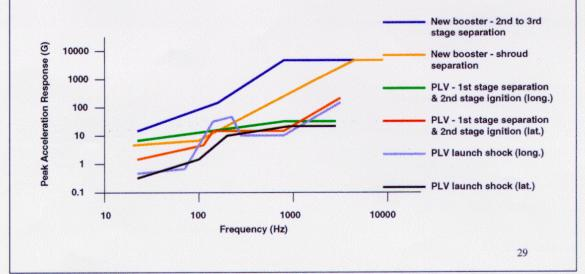
One of the highest EKV risk areas is its ability to withstand the environmental loads of the new booster that will fly on IFT-7. This chart shows that the expected shock loads are over an order of magnitude greater than those imparted from the PLV. We are not certain that the EKV will be able to withstand these loads, and we will not know with any degree of certainty until IFT-13, the flight on which the EKV and new booster are first mated together. This flight is planned for 2003.
