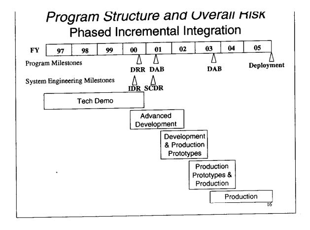
This chart provides some additional detail regarding the phased incremental approach described in the overarching observations. IDR, the Interim Design Review, is a prelude to the DRR. SCDR, the System Critical Design Review, is where the configuration of the system is fixed. The 2001 DAB is the decision to go forward with the procurement of the UEWR upgrades and the XBR. The 2003 DAB is the decision on the GBI—the final system decision.
