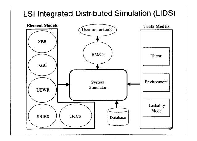
The LIDS is vital to the approach for verifying the system design. It is a simulation that includes models of the individual elements of the system and uses inputs from the threat, environment, and lethality models. It is designed to be fast-running so that it can perform thousands of runs to support the DRR. LIDS will use data from the IFTs and IGTs to verify its system descriptions.
