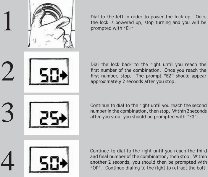
If at any time during the opening process, you are presented with a lightning bolt, you must redial the entire combination.
