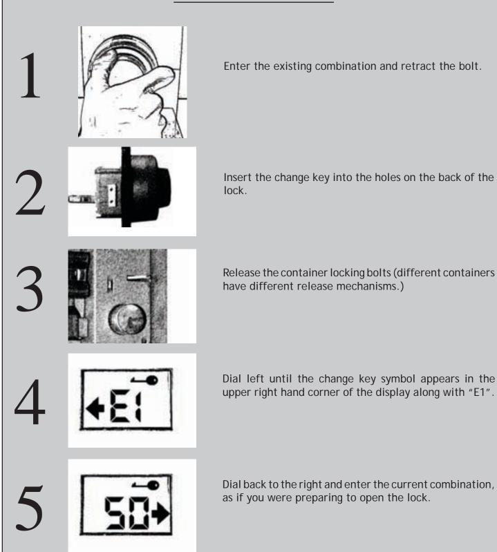
The X-08 lock is an electro-mechanical combination lock. The majority of the insides of the lock are very sensitive electronics. Under no circumstances should the owner/user remove the back plate of these locks.
