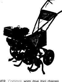
MORE POWER. Common worm drive (too) changes direction twice before it gers to the rotor At these heavy friction points. 40% of the engine's power is wasted Besides doingless work the engine wears out Sooner. The Yazoo Chain Drive (bottom) does not change direction to get to the rotor shaft There are no heavy friction points. meaning friction loss is cut by 75%. The Yazoo outperforms worm-driven machines of up to 7 HP and lasts far longer.
