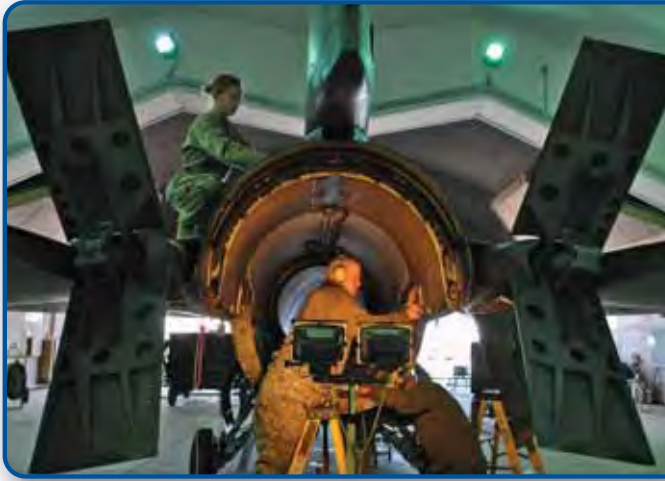
Maintenance on an F-16 Fighting Falcon at Balad Air Base, Iraq. The F-16 goes through an overhaul every 300 hours.
