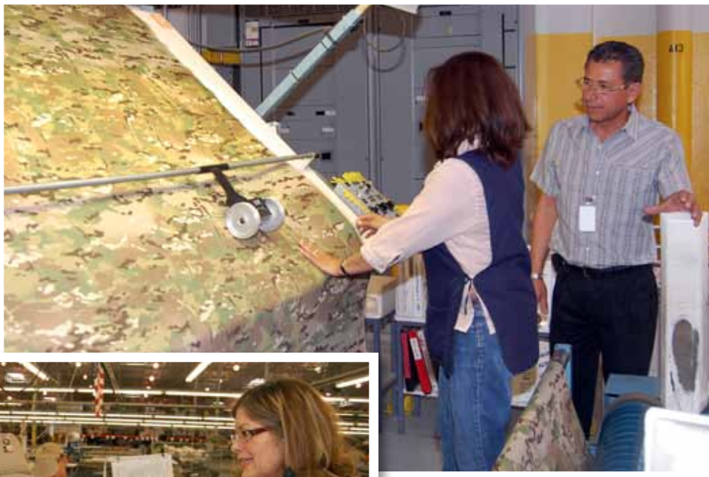
Right: Jose Arrieta, Defense Contract Management Agency quality assurance specialist, reviews the process as a ReadyOne employee inspects a large roll of uniform material. Uniform material arrives at ReadyOne Industries in rolls which must be cut down into smaller pieces before being turned into uniforms. During this stage of the process, defects are marked with a yellow piece of tape to insure they don't make it into the final product. (Photo by Matthew Montgomery, DCMA Public Affairs)
