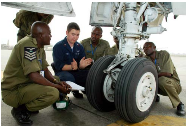
LAGOS, Nigeria — Members of the Nigerian Air Force discuss the nose-wheel steering of a P-3 Orion with Petty Officer 2nd Class Brandon Cox at Ikeja Air Force Base in Nigeria on February 25, 2008. Cox, assigned to Patrol Squadron Detachment (PATRON) Sigonella, Italy, was participating in Exercise Maritime Safari 2008, which focused on search and rescue procedures, aircraft maintenance and best practices to improve maritime safety. (Photo by U.S. Navy Petty Officer 2nd Class Jason T. Poplin)
