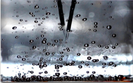
Optical probe measures bubble rise velocity and local void fraction
