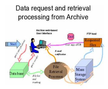
Figure 5. Data request and retrieval processing from the Data Archive.
