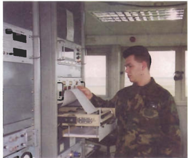
SrA. Mike Murray, an observer at RAF Mildenhall, U.K., checks wind data in the AN/FMQ-13 recorder.
